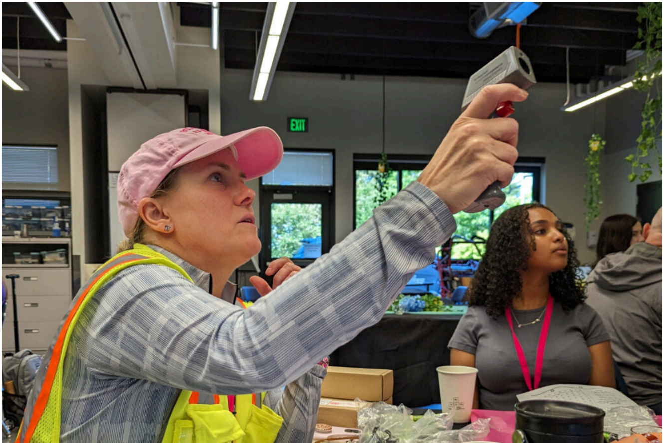
Mechanical engineer Amelia Palmer Hansen demonstrates a tool that measures the temperature at air vents.
