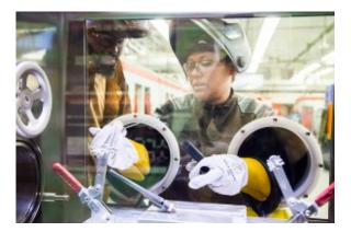
Damond Batties looks on while Nicole Doyle works in an argon purge chamber, which is used in welding air-sensitive materials like stainless steel and titanium that are common in modern industry.
